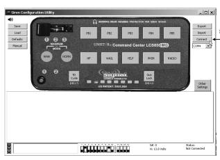
The interface will open. Press the **Connect** button on the right side or the window to connect the Siren Configuration Utility to the siren. It should automatically detect the correct COM port.
